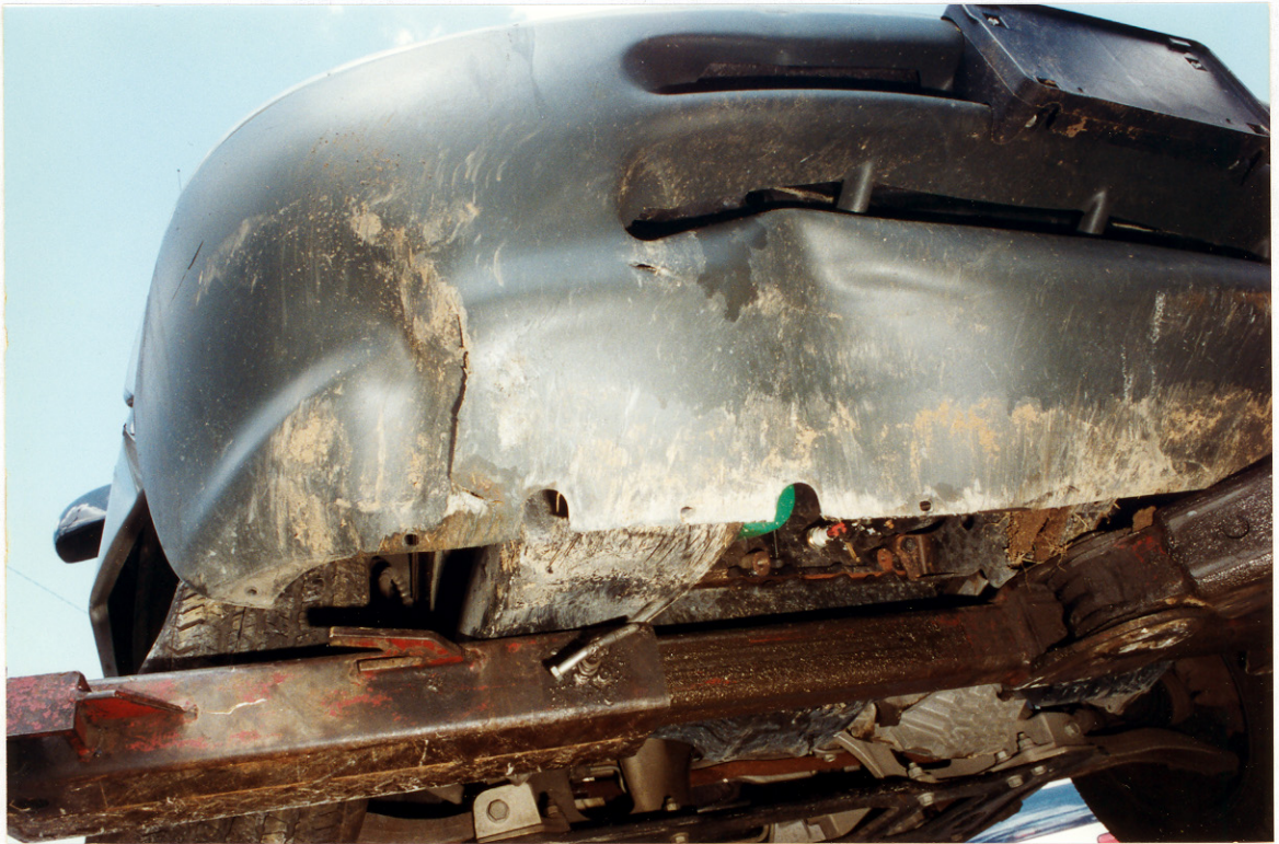
36. Close up view of damage to the lower surface of the bumper fascia.
